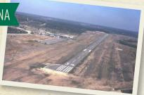
The airport is located one mile north of Ozona. In 1998, a \$2.4 million federal grant was used to upgrade the runway, taxiway, and lighting system. The all-weather hot mix asphalt runway is 6,000 feet in length, 75 feet wide, and will accommodate any aircraft weighing up to 70,000 lbs. There is a very large parking area and radio-controlled lights for strong illumination. G.P.S. IFR Approach OZA (KOZA)
